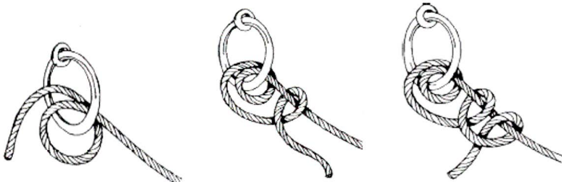
CFCD 105 Seamanship Rigging and Procedures Manual Figure 10-1-6 Round Turn and Two Half Hitches
